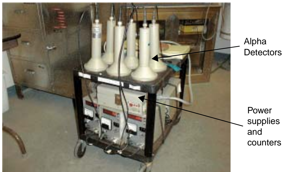
Figure 6. Multiple alpha detector and scalar array: The sample and reference filters containing radon-progeny labeled particles collected in tests of the virtual impactor are simultaneously counted in an array of ZnS(Ag) alpha-scintillation detector/scalar counters.
