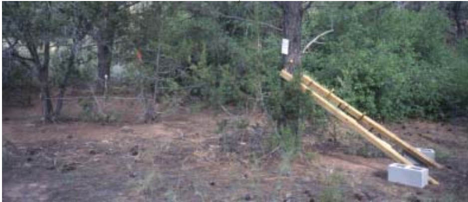
Figure 1. Two types of hair snares are shown. The cubby snare (right) grabs hair samples from animals entering the snare to investigate scents that are placed on the tree. Hair is taken from animals using a series of brushes placed along the two timbers. The barbed wire snare (left) grabs hair samples from animals entering the enclosed area (scents are placed at the center of the area to attract animals). The barbs are long enough to grab hair without injuring the animal.
