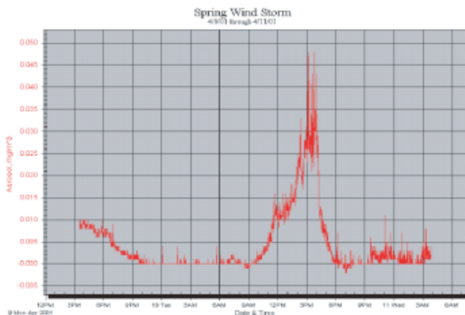
Figure 5. One-minute PM-10 aerosol concentrations taken at the TA-6 burned area during a wind storm.
